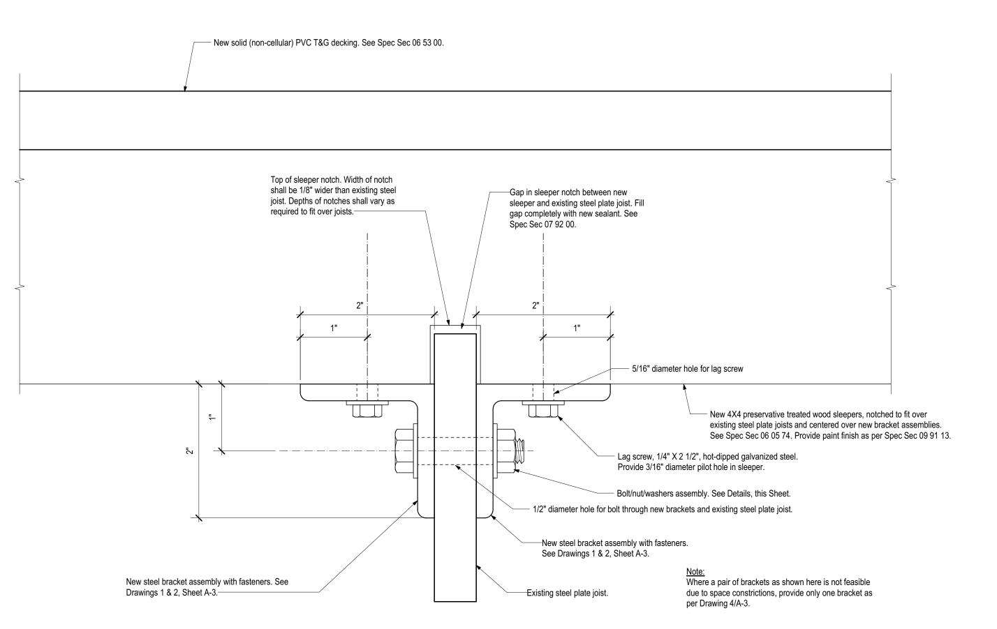
6 Detail: Section at Typical Bracket Assembly (Two Brackets)
